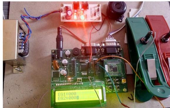
**Liquid-crystal display (LCD)** is a flat panel display, electronic visual display that uses the light modulation properties of liquid crystals. Liquid crystals do not emit light directly. LCDs are available to display arbitrary images or fixed images which can be displayed or hidden, such as preset words, digits, and 7-segment displays as in a digital clock.
