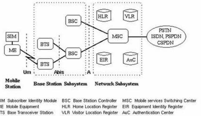
Fig: GSM architecture
