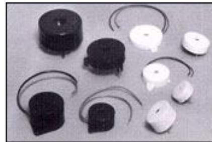
FIG: Types of Buzzers
