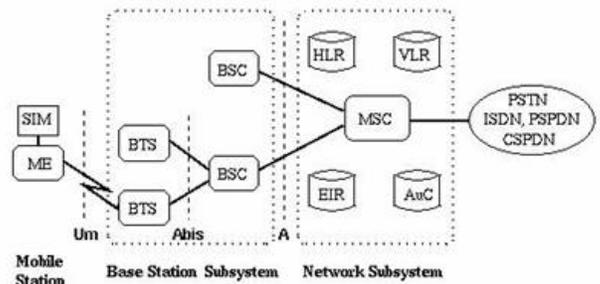
SIM Subscriber Identity Module    BSC Base Station Controller    MSC Mobile services Switching Center
