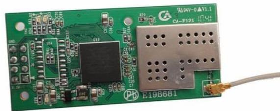
VSD03 is the new third-generation embedded Uart Wifi modules studied by VSDTECH. Uart-Wif is an embedded module based on the Uart serial,according with the WiFi wireless WLAN standards, It accords with IEEE802.11 protocol stack and TCP / IP protocol stack, and it enables the data conversion between the user serial and the wireless network module. through the Uart-Wifi module, the traditional serial devices can easily access to the
