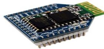
AUBTM-22 is a Bluetooth v1.2 module with SPP profiles. The module is intended to be integrated into another HOST system which requires Bluetooth functions. The HOST system could send commands to AUBTM-22 through a UART. AUBTM-22 will parse the commands and execute proper functions, e.g. set the maximum transmit power, change the name of the module. And next the module can transmit the data receive from the uart with SPP profiles.
