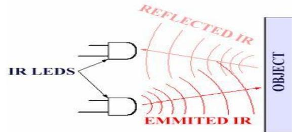
Fig.4.Eye Blink Sensor(IR Led's)
