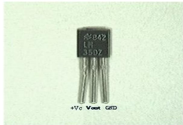
It has an output voltage that is proportional to the Celsius temperature. The scale factor is  $.01V/°C$  The LM35 does not require any external calibration or trimming and maintains an accuracy of  $\pm 0.4 °C$  at room temperature and  $\pm 0.8 °C$  over a range of  $0 °C$  to  $+100 °C$ . Another important characteristic of the LM35DZ is that it draws only 60 micro amps from its
