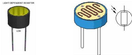
The output of the LDR is given to ADC which converts the analog intensity value into corresponding digital data and presents this data as the input to the microcontroller
