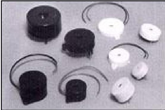
Fig 3: Types Of Buzzers
