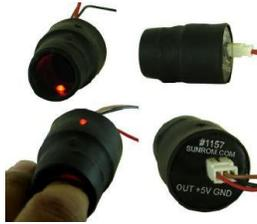
Fig 4 .Pulse sensor
