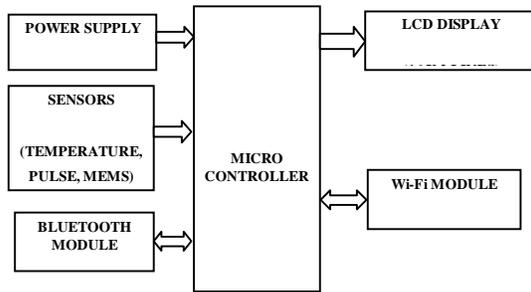
Fig 1. Block diagram for Transmitter
