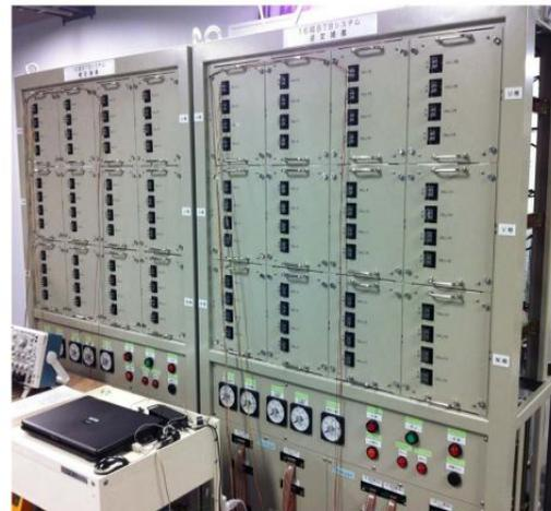
Fig.4. Photo of the three-phase 200-V, 10-kW, 50-Hz BTB system used for experiment.
