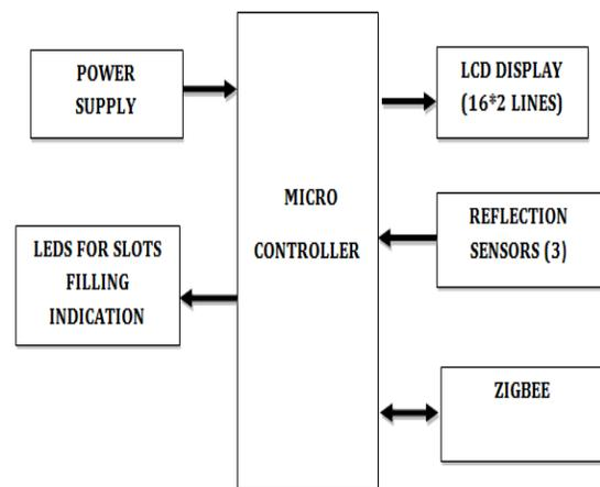
**Fig: Parking Section Block Diagram**
