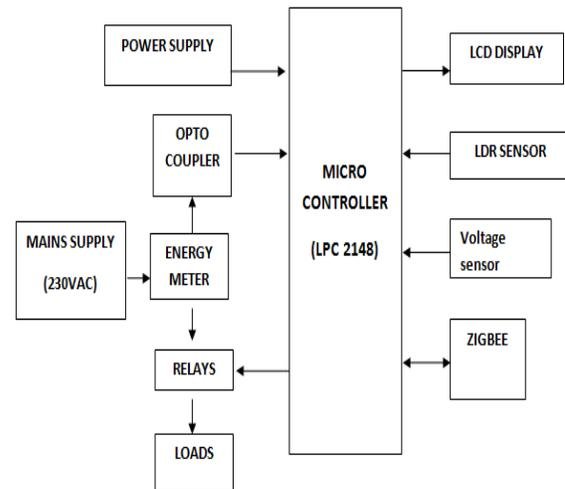
Fig.1. Field Section Block diagram
