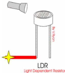
LDRs or Light Dependent Resistors are very useful especially in light/dark sensor circuits. Normally the resistance of an LDR is very high, sometimes as high as
