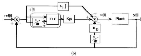
**Fig 2 Control schemes (a) PID-type controller. (b) Fuzzy P+ID controller**
