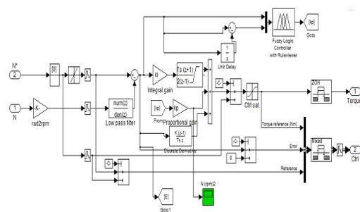
**Fig 8(b) Subsystem of speed controller of PMSM HFLC**
