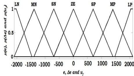
**Fig: 4 Membership function for error, change in error and fuzzy**
