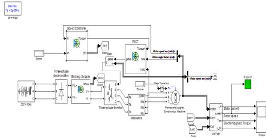
**Fig.8 (a) PM Synchronous Motor drive subsystem**
