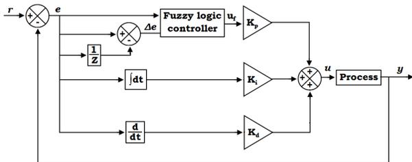
**Figure 3 Hybrid PID Fuzzy Logic Controller**
