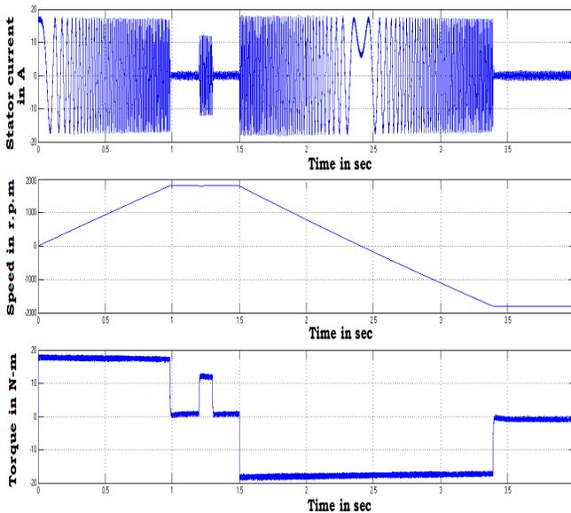
**Fig.9 Dynamic response of PMSM during starting, load perturbation and speed reversal at 1800 r.p.m with PI controller**
