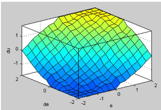
Fig6. Control surfaces of the incremental fuzzy logic controller
