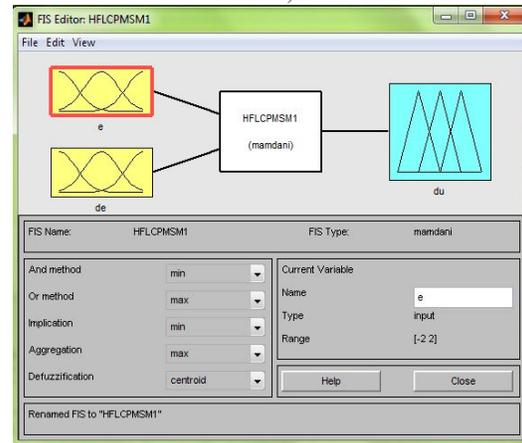
**Fig.8 (c) FIS editor of PM Synchronous Motor speed control**
