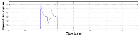
**Fig 10 Magnified view of speed response of PMSM during starting and load perturbation at 1800 r.p.m with PI controller**
