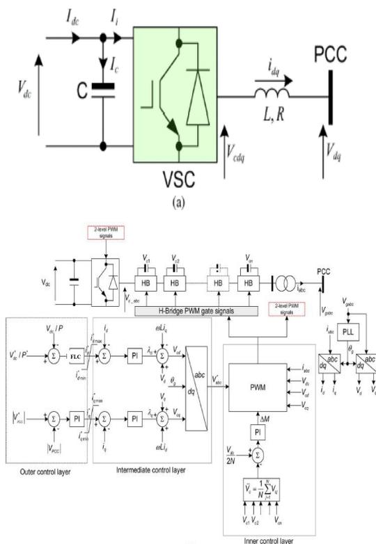
Fig. 2. (a) Representation of VSC station and (b) schematic diagram summarizing the control layer of the hybrid multilevel converter with ac side cascaded
