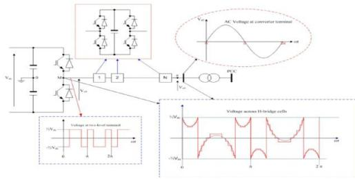
Fig. 1. Hybrid voltage multilevel converter with ac side cascaded H-bridge cells
