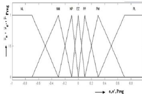
Fig. 4. Memberships function for the input and output variables.
