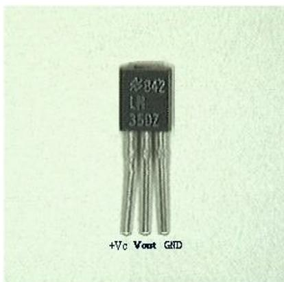
Fig.4. Temperature sensor
