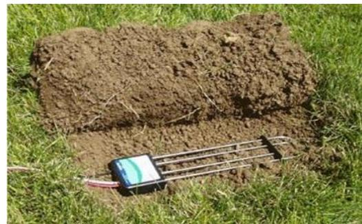
**Fig.4. Soil Sensor**
