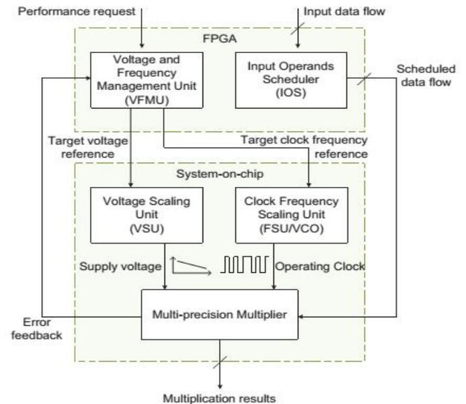
Fig.1: Overall multiplier system architecture.
