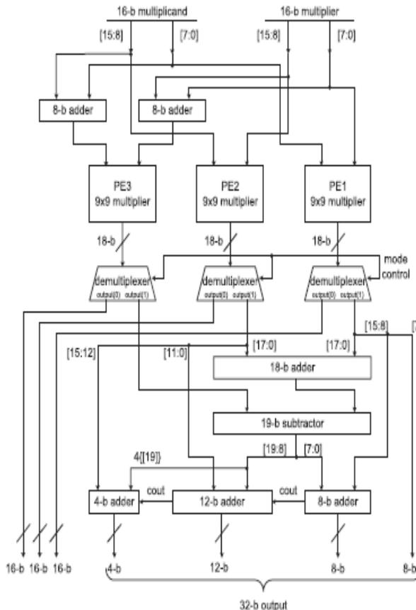
Fig.3 : Three PEs combined to form 16 x 16 bit multiplier
