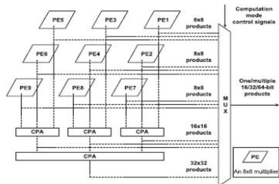
Fig.2: Possible configuration modes of existing MP multiplier
