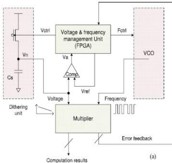
Fig.4: Proposed single-header voltage dithering unit
