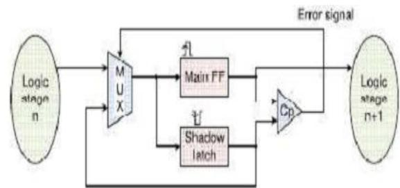
Fig.5: Conceptual view of razor flip-flops
