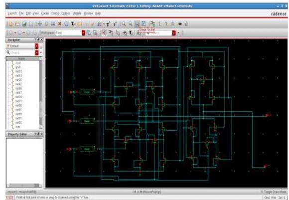
Figure 1.2: Schematic of bridge Full Adder
