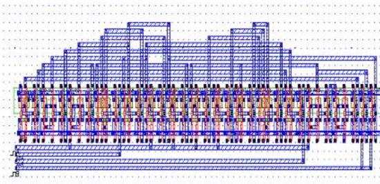
Fig.10. layout design of proposed full adder based comparator
