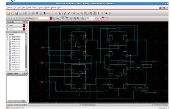
Figure 2.3: Schematic of FA24T Full Adder in cadence tool
