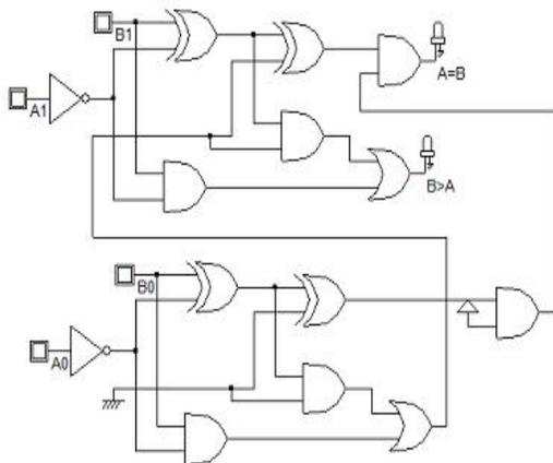
Fig.3.Logic diagram of basic full adder comparator
