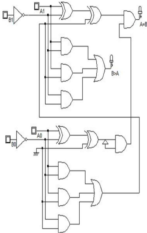
Fig.6 logic diagram of proposed full adder based comparator
