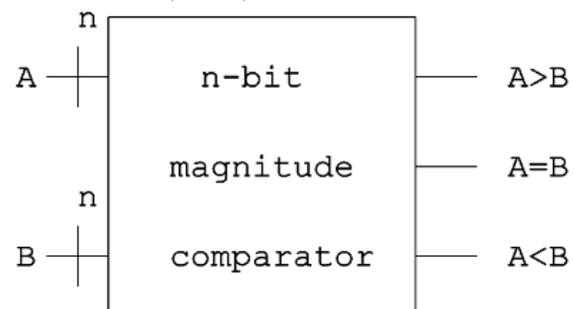
Figure 1.1: block diagram of n-bit magnitude comparator
