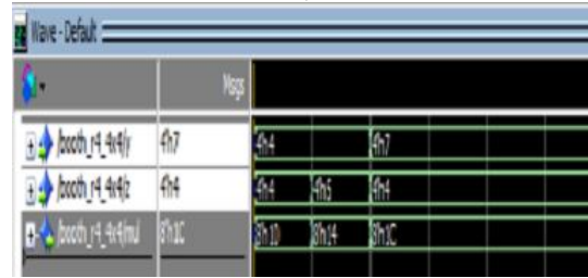
Figure 9. 8x8 bit Modified Booth Multiplication using ModelSim
