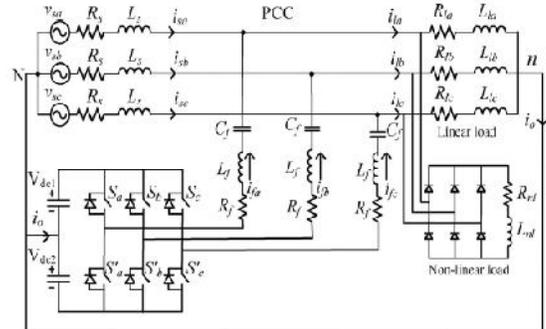
Fig. 2. Equivalent circuit of the proposed neutral clamped VSI topology-based DSTATCOM (hybrid filter).
