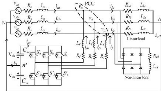
Fig. 1. Equivalent circuit of the neutral clamped VSI topology-based DSTATCOM.
