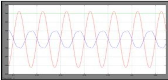
Fig. 6. Voltage across top dc capacitor, series filter capacitor, and terminal voltage in phase-*a*.
