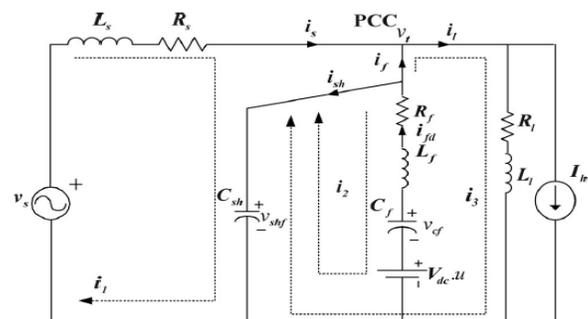
Fig. 3. Single-line diagram of the proposed DSTATCOM.
