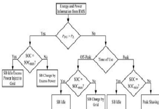
Fig. 2. Operation of the SB during grid-connected operation. [10], and the output voltage of the PV array is permitted to vary within an allowable range to ensure proper operation of the DG inverter. To maintain the level of the
