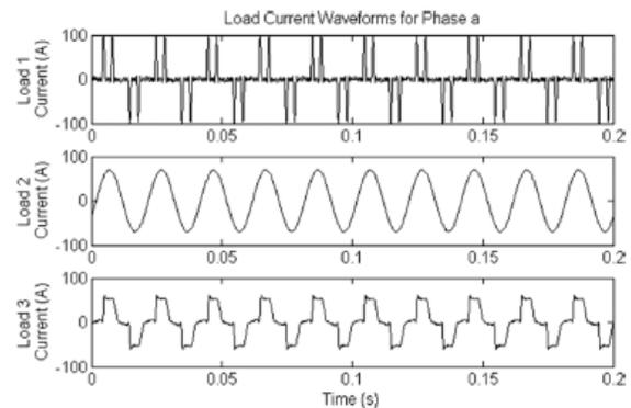
Fig. 9. Per-phase currents drawn by loads 1, 2, and 3.
