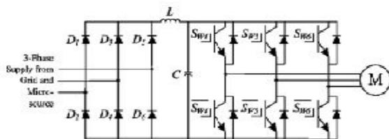
Fig. 8. Configuration of a 15-kVA three-phase ASD.
