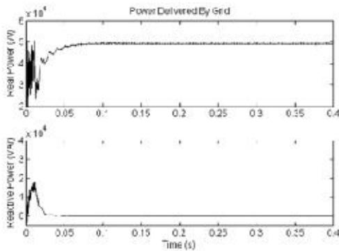
Fig. 16. Real (top) and reactive (bottom) power delivered by the grid.
