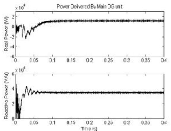
Fig. 15. Real (top) and reactive (bottom) power delivered by the main DG unit.
