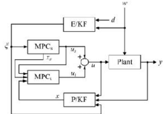
Fig. 7. Overall MPC controller for the DG inverter with E/KF denoting the exogenous Kalman filter and P/KF denoting the plant Kalman filter.
