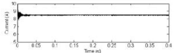
Fig. 10. Waveform of the SB current during charging.
