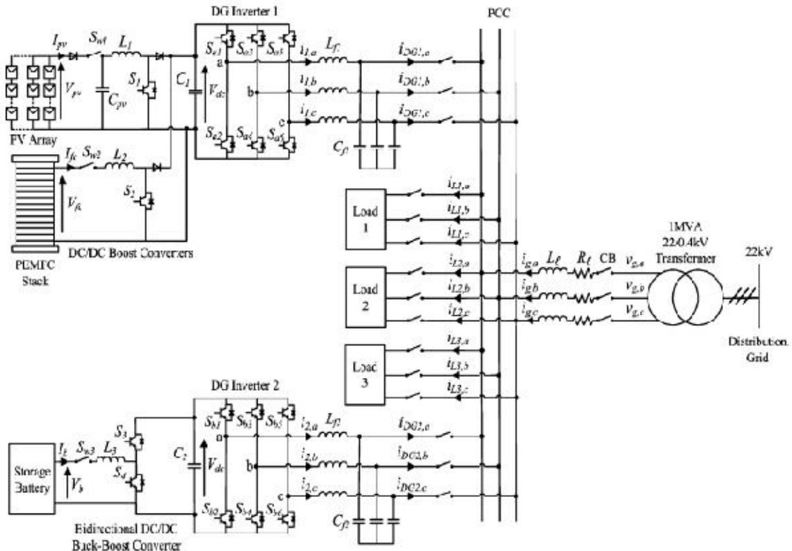
Fig. 1. Overall configuration of the proposed microgrid architecture
