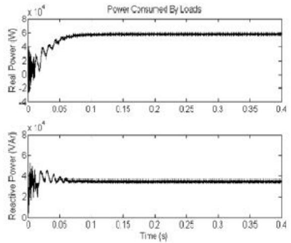
Fig. 14. Real (top) and reactive (bottom) power consumed by loads.
