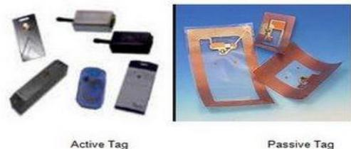
Active tags require a power source i.e., they are either connected to a powered infrastructure or use energy stored
