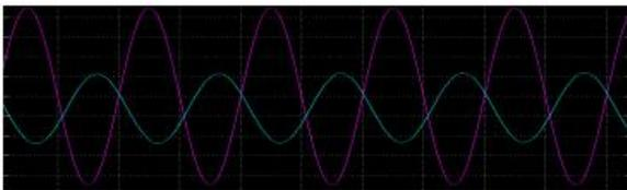
Fig 11. Grid voltage and grid-connected current
